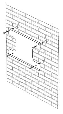
3. First check the 4 holes in the backside of the inverter. Then, lift the inverter carefully, align the 4 holes in the inverter and the 4 screws in the wall, and finally attach the inverter to the screws slightly.
