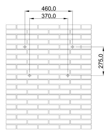
2. First, according to the marks, drill 4 holes in the wall. Then, place four expansion tubes in the holes using a rubber hammer. Next, wring 4 screws into the expansion tubes.
